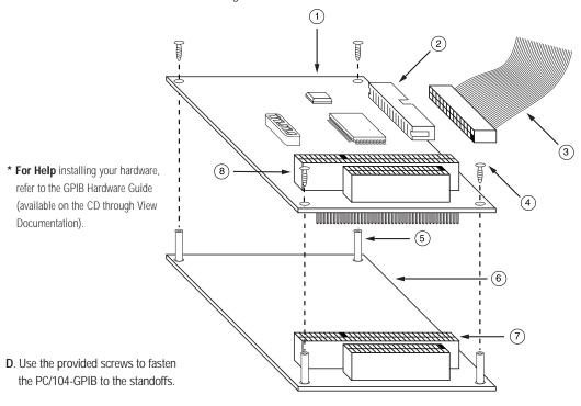
E. Plug in the GPIB ribbon cable.
